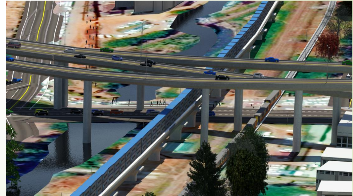
Harmonized SGR-Flyover at Access Road Level.
